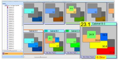
**Active Facility Maps:** Create accurate facility maps to mimic data center layouts and get detailed information down to the cabinet level including 3D temperature maps, rack and device level power consumption and more.
