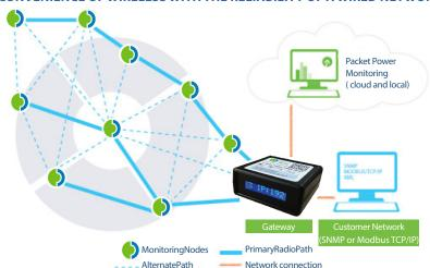
Packet Power's self configuring mesh network delivers all the advantages of wireless connectivity while eliminating the traditional difficulties associated with wireless propagation and system configuration. If a direct connection to the Gateway is not optimal, the system routes the data through other monitors, optimizing each path with every transmission.
