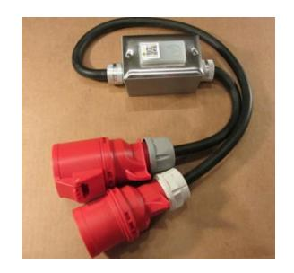
Smart Power Cord with in-line wireless power monitoring. IEC 60309 532P6S plug and 532C6S connector. For use on a 32A, 240/415V 3ØY circuit with circuit protection.
